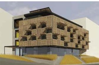
Pallets Building This project is to finish a building that currently stands as a concrete structure. A new facade from recycled wooden pallets will shade the interior. Some of the pallets are designed to open and close electrically, so as to provide with sea views. At ground level there are shops and common areas, while the upper floors will accommodate office space.
